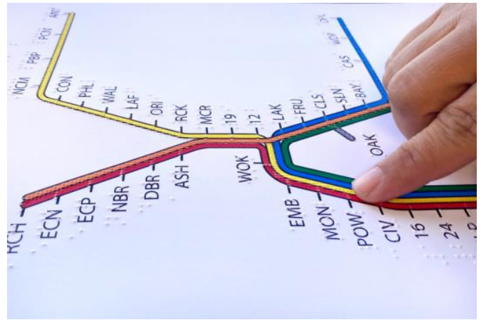
Figure 2. Finger on tactile BART system map, an embossed paper product with raised lines, braille labels, and full-color graphics.
